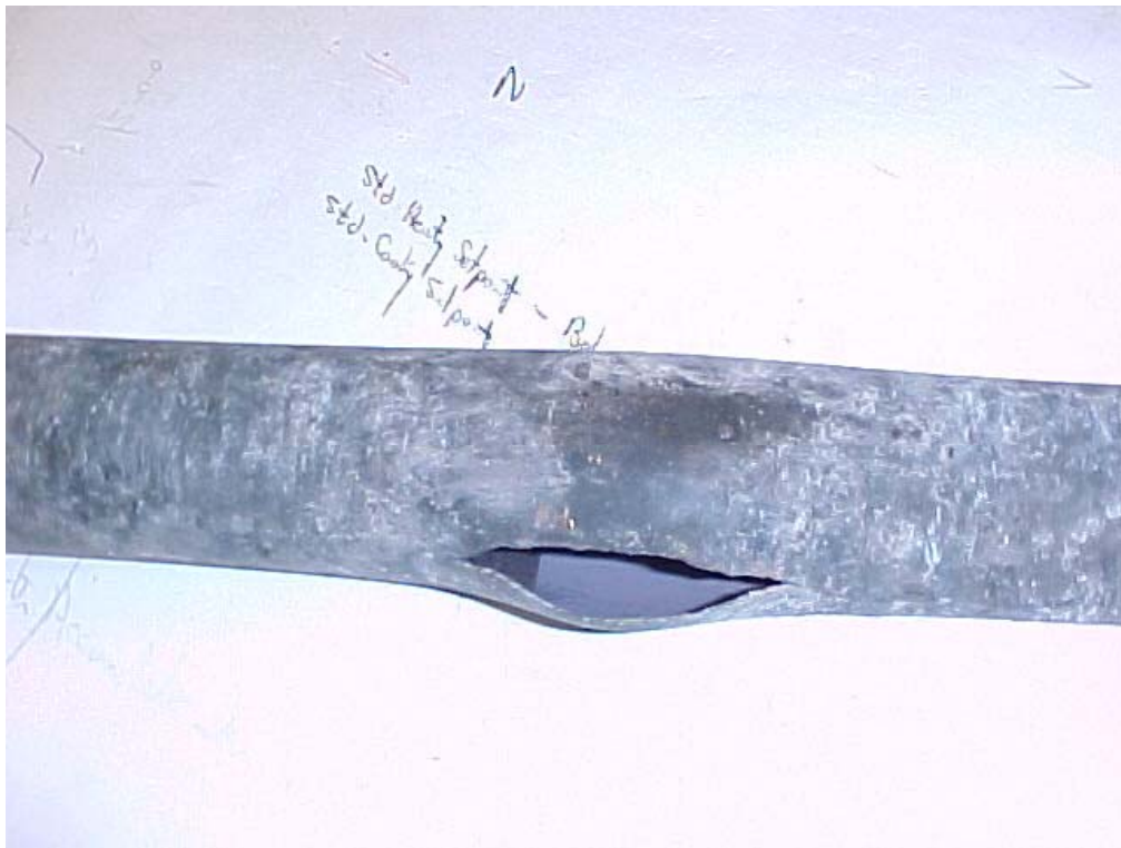
Ruptured steam tube
