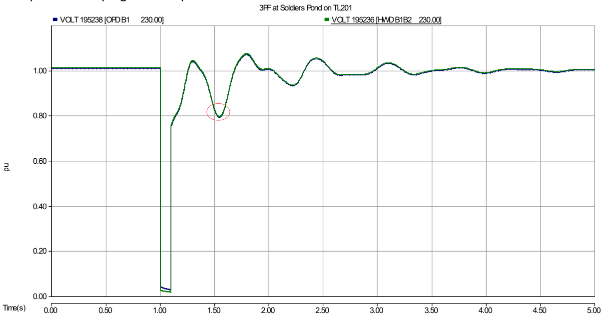
Figure 5-2. 230 kV voltage at Oxen Pond and Hardwoods for 3PF TL201 at Soldiers Pond.
