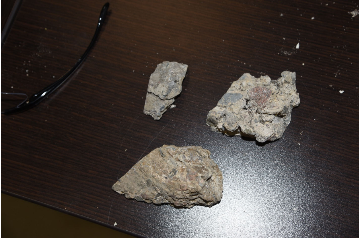
Small Pieces of Concrete found on the Lower Platform
