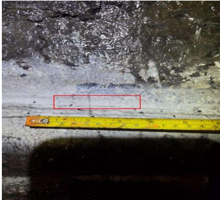
Figure 5. Can 35 North - Indication #3 - Intermittent Indication Noted
