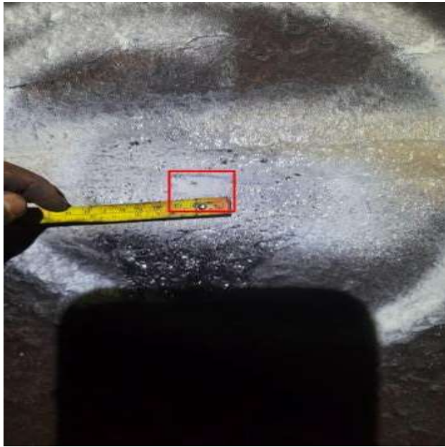
Figure 16. Can 263 South - Indication Noted - Post Grinding
