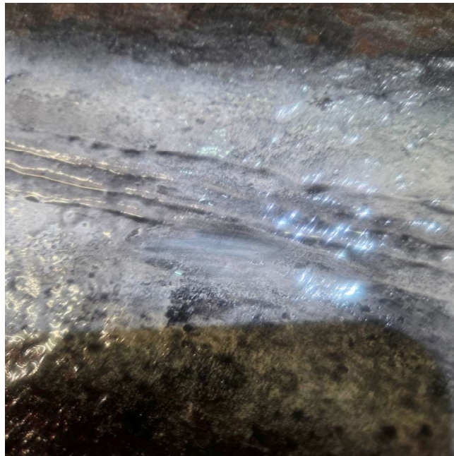
Figure 20. Can 322 North - Post Grinding - Indication Removed
