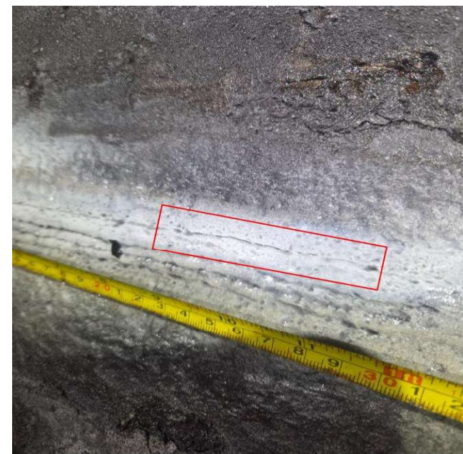
Figure 9. Can 77 South - Indication #5 Intermittent Indication Noted
