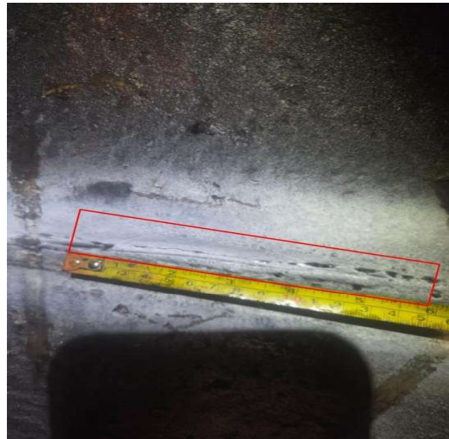
Figure 9. Can 77 South - Indication #5 Intermittent Indication Noted
