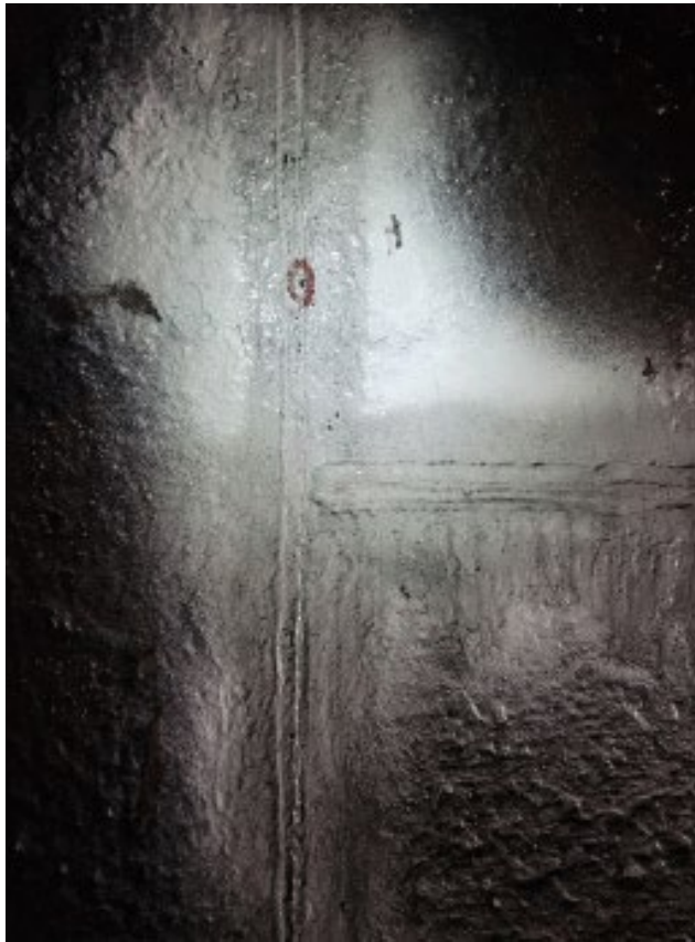
Photo 12 Indication in Circumferential Weld,;Can 98
