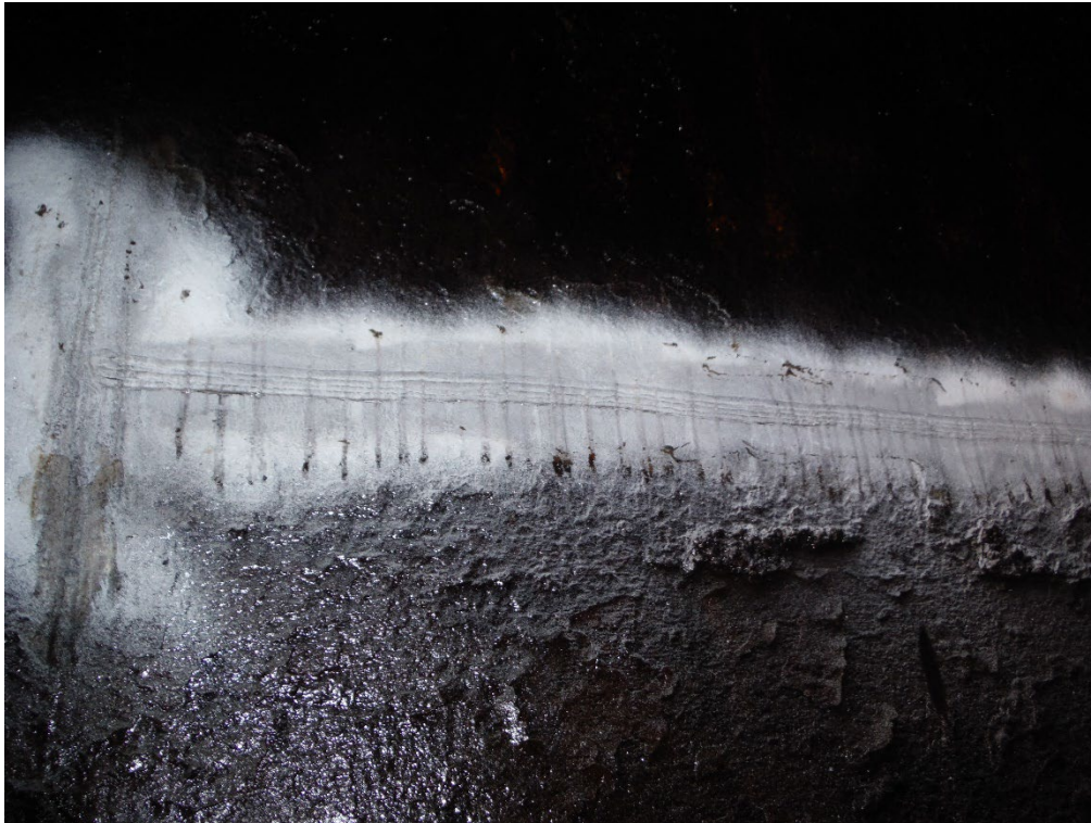
Photo 9 Previously repaired weld retested; Typical Condition
