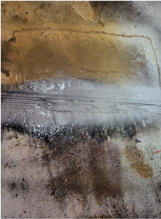
Figure 3. 145N Weld Repaired - Checked at 11:15 AM April 28 th 2022 (Post Welding)
