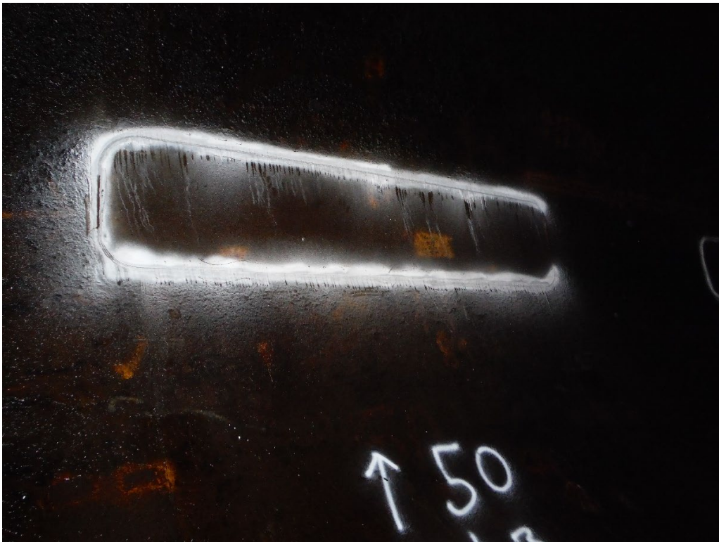
Photo 8 Plate repair welds tested. Can 50
