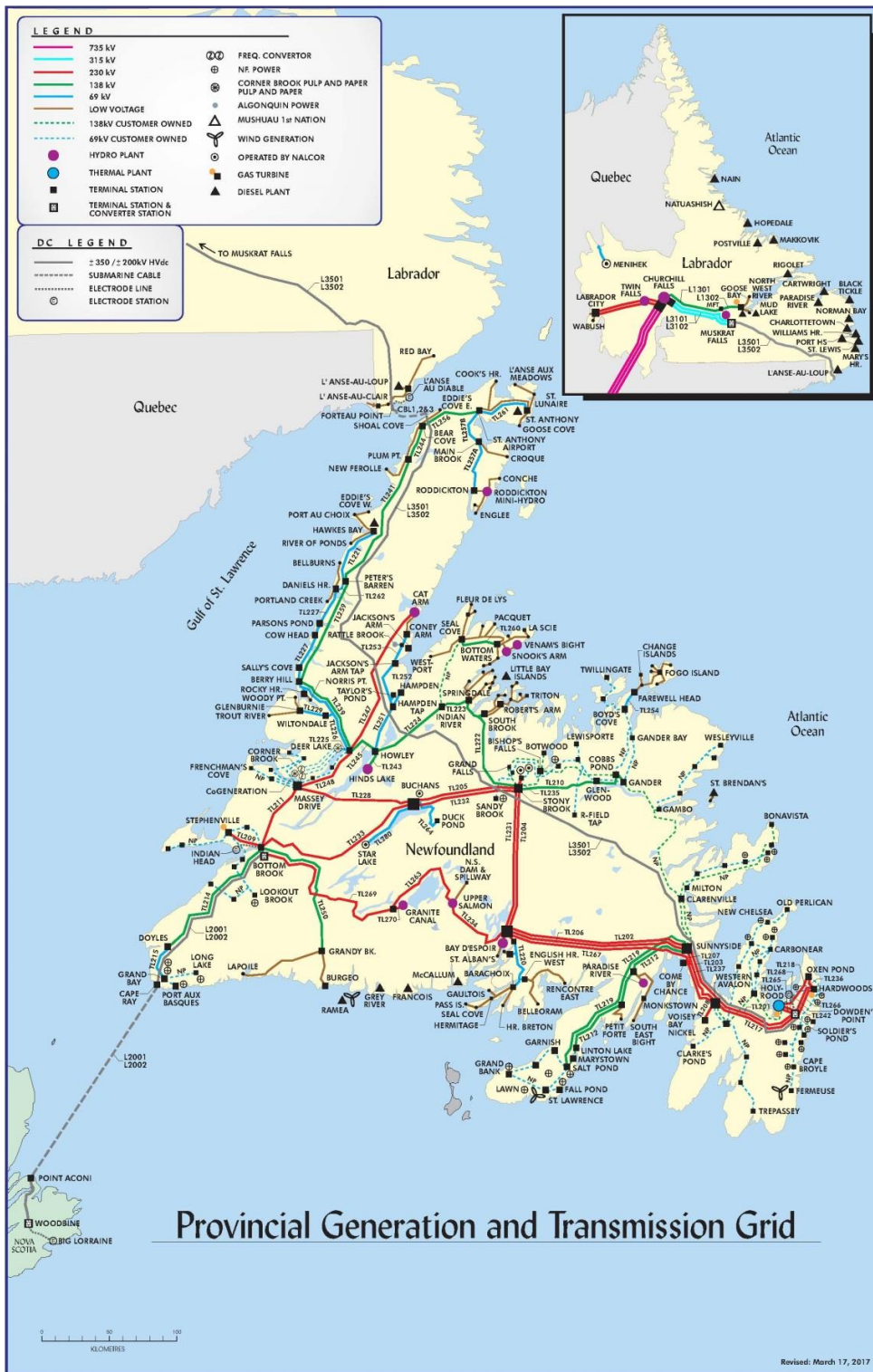
Figure 1 –Newfoundland and Labrador Interconnected System
