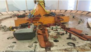
Figure 1 – Leads with brackets removed and additional insulation placed beneath them
