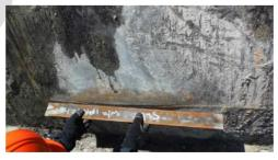
Figure 3-2: Longitudinal Weld Failure Showing Peaking
