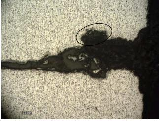
Figure 6: Microscopic Views of Typical Tube Internal Cracks. Variation in Crack Width is Evident. Occluded Pits Are Circled. Corrosion Product Is Visible Within Cracks.
