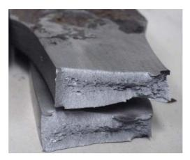
Figure 8-3: Ductile Failure Tensile Tests Penstock No. 1
