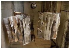
Figure 1 - Connection broken between poles 15 and 16
