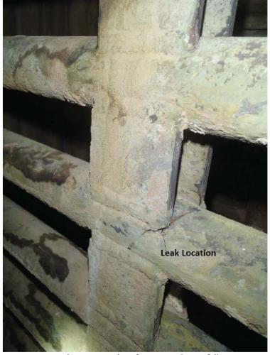
Figure 2: Location of LTSH attachment failure
