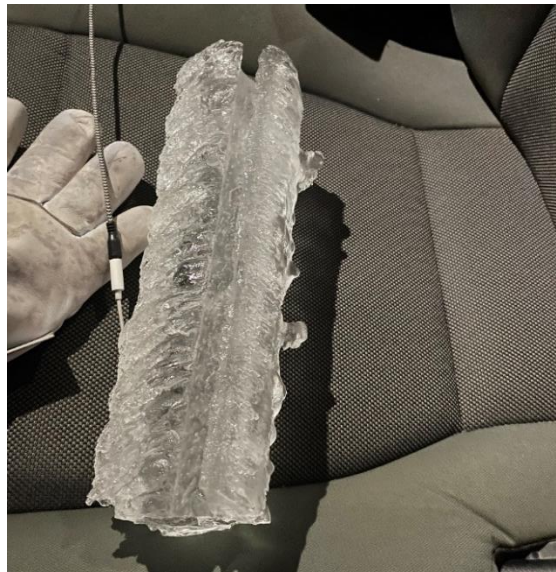
Figure 8: Ice Sample from the Distribution Line in Red Bay
