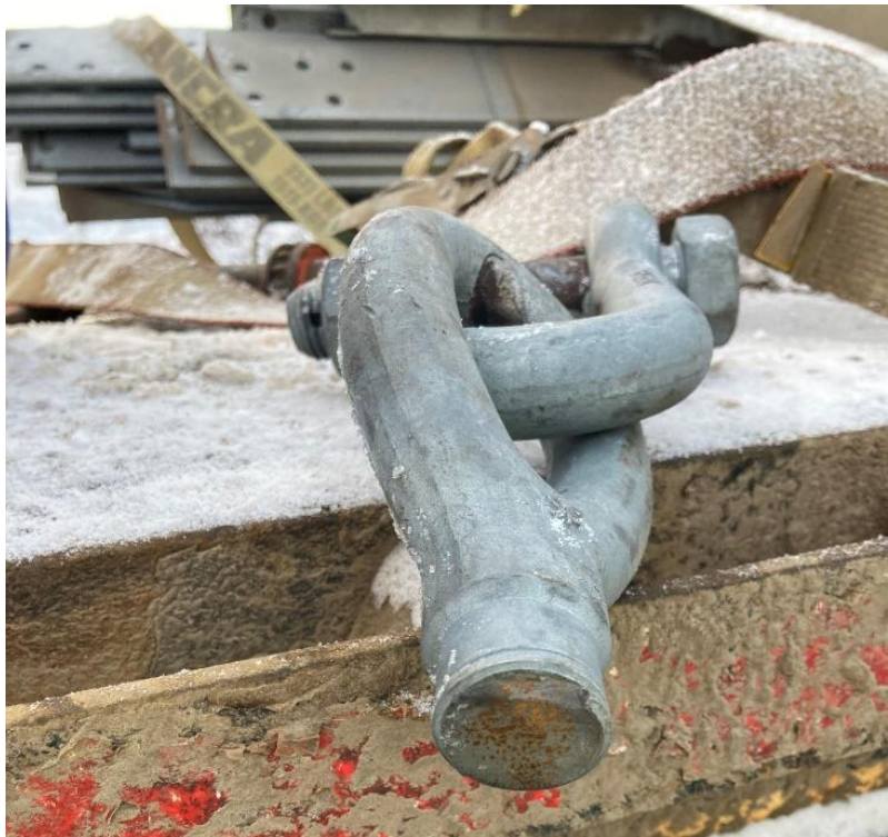
Figure 5: Failed Turnbuckle Eye and Shackle
