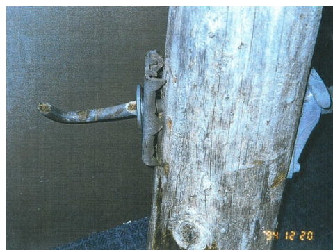
Figure 8.3 (a) Figure 8.3 Bridge Failure of a Guyed-V Suspension Tower in 1988 (b) Large Angle Tower Failure near Hawke Hill (1988 Storm) (c) aa glaze ice sample during 1984 storm on the Avalon Peninsula and (d) Failure of a Forged Eye Bolt in 1994
