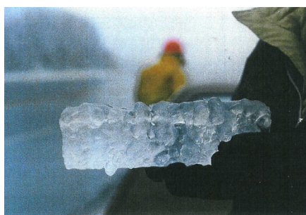
Figure 8.3 (a) Figure 8.3 Bridge Failure of a Guyed-V Suspension Tower in 1988 (b) Large Angle Tower Failure near Hawke Hill (1988 Storm) (c) aa glaze ice sample during 1984 storm on the Avalon Peninsula and (d) Failure of a Forged Eye Bolt in 1994
