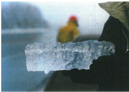
Figure 8.3 (a) Bridge Failure of a Guyed-V Suspension Tower in 1988 (b) Large Angle Tower Failure near Hawke Hill (1988 Storm) (c) aa glaze ice sample during 1984 storm on the Avalon Peninsula and (d) Failure of a Forged Eye Bolt in 1994
