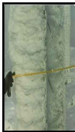
963 964 Figure 4.4 Observed Rime Icing in Labrador 965
