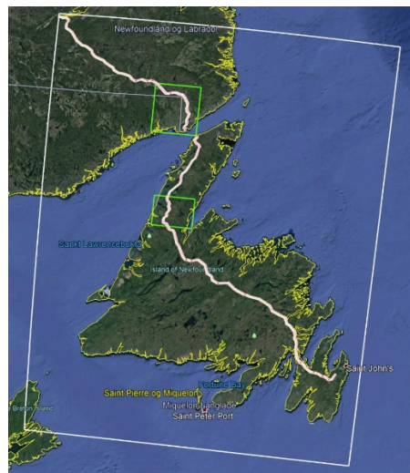
1023 1024 Figure 4.6 Setup of the WRF model simulations (The WRF4km domain is shown as the white 1025 rectangle and the two green rectangles show the two WRF500m domains) –EFLA (2021)
