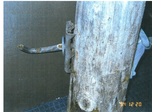
Figure 8.3 (a) Bridge Failure of a Guyed-V Suspension Tower in 1988 (b) Large Angle Tower Failure near Hawke Hill (1988 Storm) (c) aa glaze ice sample during 1984 storm on the Avalon Peninsula and (d) Failure of a Forged Eye Bolt in 1994
