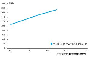
Assumptions One wind turbine, 100% availability, 0% losses, k factor -2, Standard air density - 1.225, wind speed at hub height
