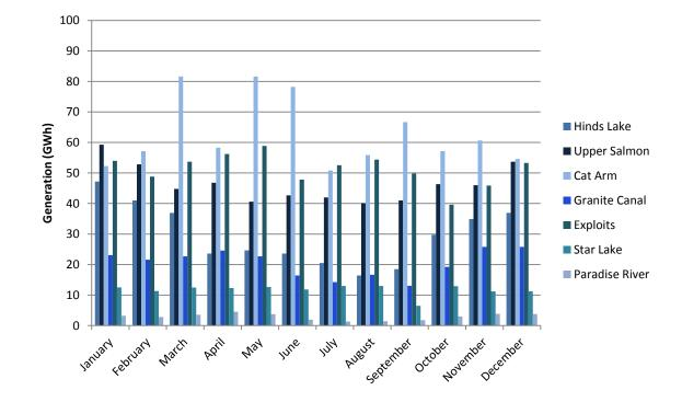
1 Figure 3 shows the energy profiles modeled for other hydraulic generation in the system.
