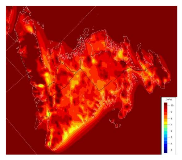
Figure 2: Estimated average annual wind speed at 80m hub height (courtesy <u>www.windatlas.ca</u>)
