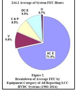
Figure 3: Breakdown of Average FEU by Equipment Category (LCC)<sup>6</sup>
