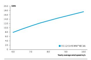
Assumptions One wind turbine, 100% availability, 0% losses, k factor =2, Standard air density = 1.225, wind speed at hub height
