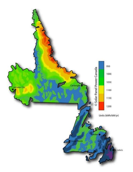
Figure 2: High level solar resource for NL (courtesy of Solar Panel Power Canada). Note, darker blue and purple colours (e.g. Avalon Peninsula) have capacity ratios lower than 950 kWh/KW/yr.
