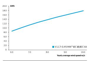
$\label{eq:sumptions} \begin{array}{l} \text{Assumptions} \\ \text{One wind turbine, } 100\% \text{ availability, } 0\% \text{ losses, } k \text{ factor = 2,} \\ \text{Standard air density = } 1.225, \text{ wind speed at hub height} \end{array}$
