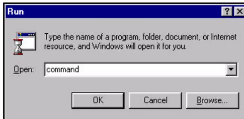
3. At the command line prompt, enter 'ping IP Address of the XMU+'. 'IP Address of the XMU+' is the IP address assigned to the XMU+ in *Assigning and Testing IP addresses* on page 98.
