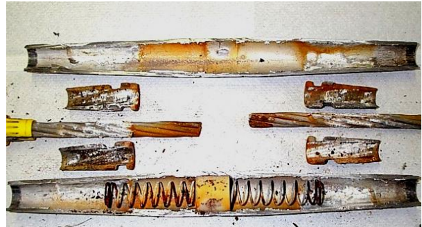
Figure 10: Disassembled Automatic Sleeve Showing Corrosion
