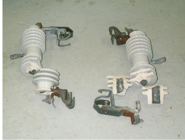
Figure 12: Two Broken Porcelain Cutouts Removed From Service
