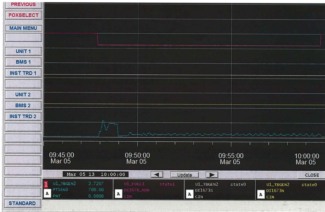
Figure 2: DC lube oil pump test from March 5, 2013. Note the falling magenta line indicates starting of the DC lube oil pump. There is an increase in pressure (blue) for a short time before pressure crashes and cycles
