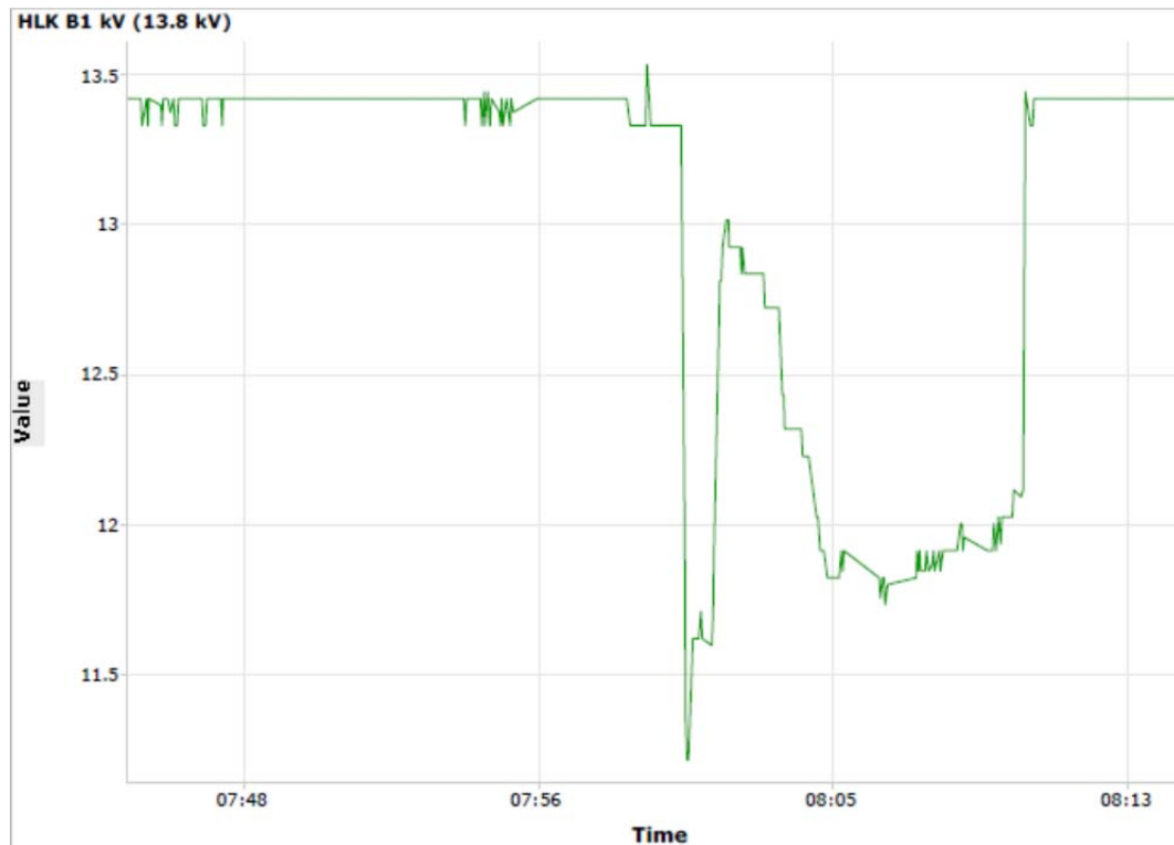
Figure 3-9a: Hinds Lake Terminal Voltage from 0745 to 0815 Hours
