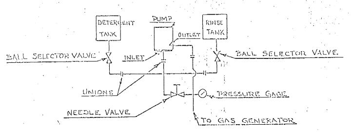
PLUMPING SCHENATIC. GENERATOR COMPRESSOR WASH - GAS TIQUID
