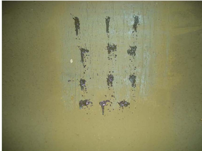
Figure 3-6: Interior of Tank Bowl with UT Couplant
