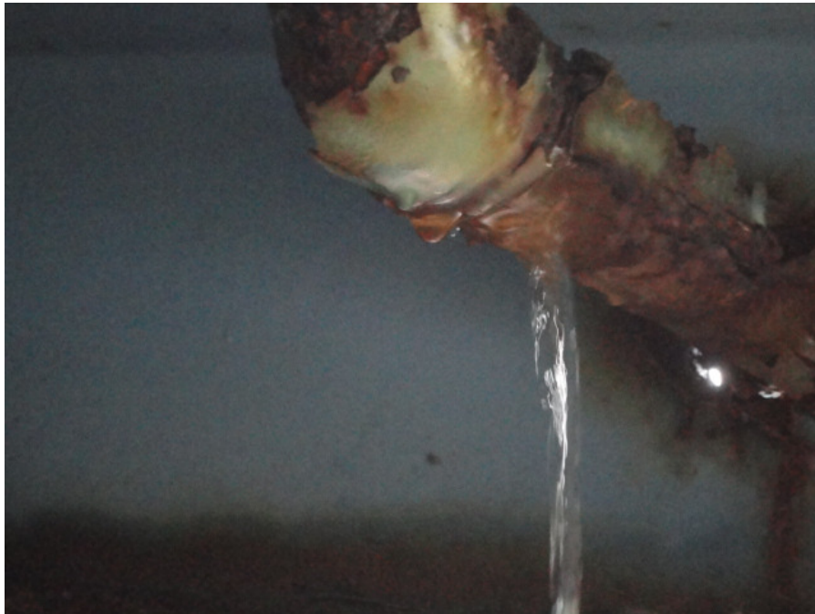
Figure 2: Water Leaking from Dyke Drain Valve Piping During Leak Test
