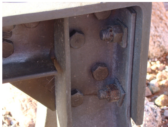
Figure 6: Failed Bolt Connection on Structure 216 of TL206
