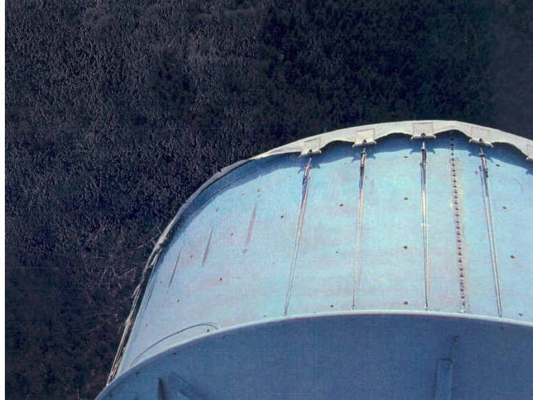
Figure 4: Missing Radome Mounts
