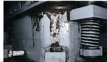
HEAVY COLLECTION OF OIL AND BREAK PADS DUST OVER CYLINDERS OF THE BRAKING SYSTEM
