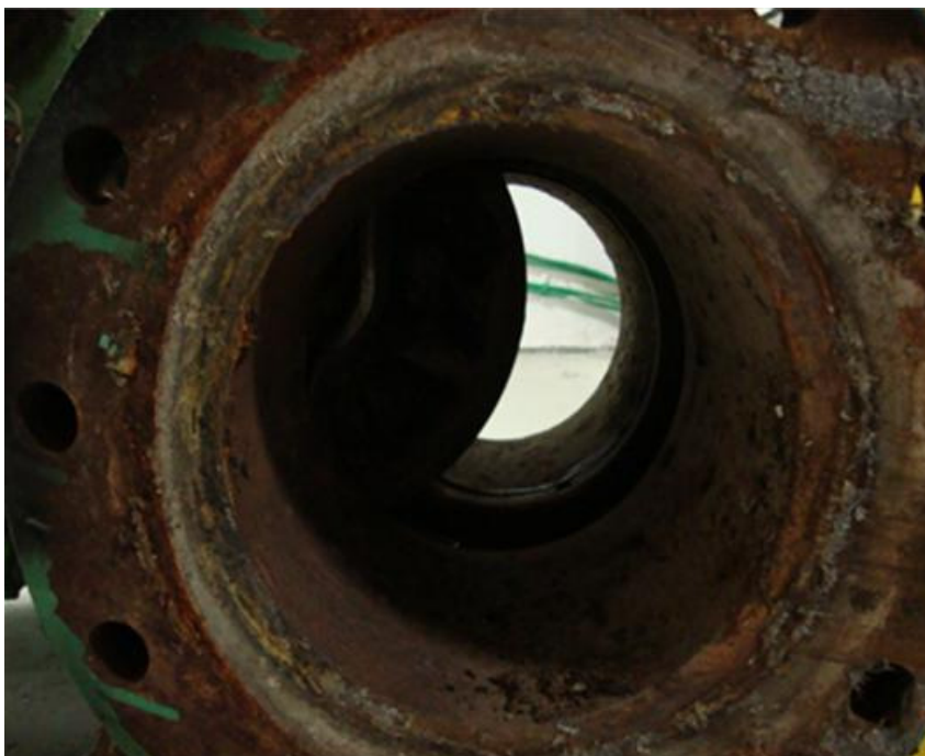
Figure 2: By-Pass Valve with Disk Jammed in Half Open Position
