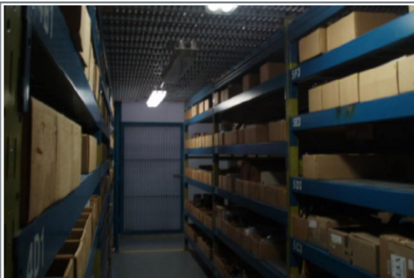
Sprinklers are needed below the grated mezzanine in the Main Warehouse.
