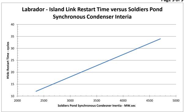
Given that the project now includes three 175 MVAR high inertia synchronous condensers, the SNC-Lavalin results indicate that with two 175 MVAR synchronous condensers in service with a total inertia contribution of 2744 MW.sec, one expects the maximum restart time for the temporary bipole failure to be approximately 15 cycles or 250 msec. With three 175 MVAR synchronous condensers in service at Soldiers Pond (4116 MW.sec) the maximum restart time is estimated to be 28 cycles or 467 msec.
