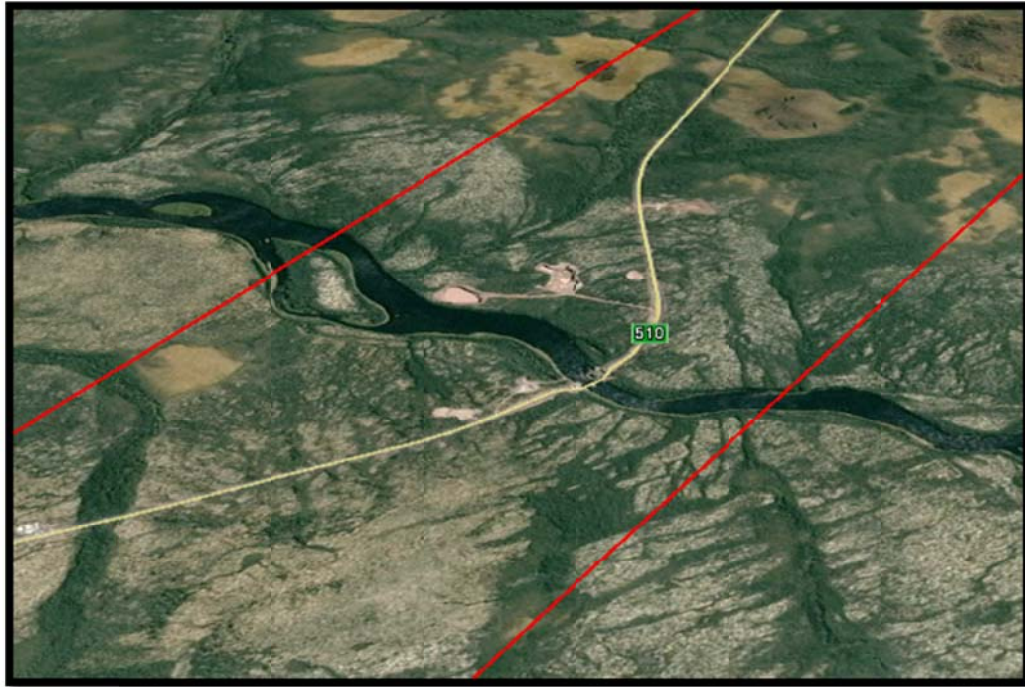
Figure 7: Typical river and highway crossings along the HVdc transmission line route. Crossing spans are achievable with the current transmission line design parameters.
