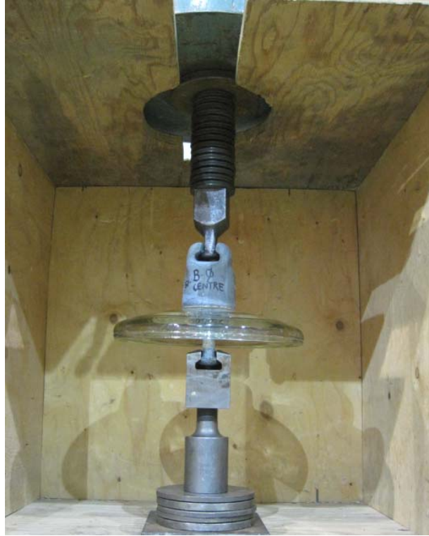
Figure 2 Insulator Sample Prepared for Mechanical Testing
