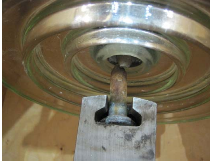
Figure 6 Typical Insulator Sample after Mechanical Test (failed at Pin Base)
