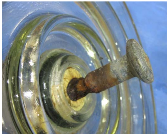
Figure 7 Typical Insulator Sample as received, Bottom View, Magnified View of Pin with Severe Corrosion
