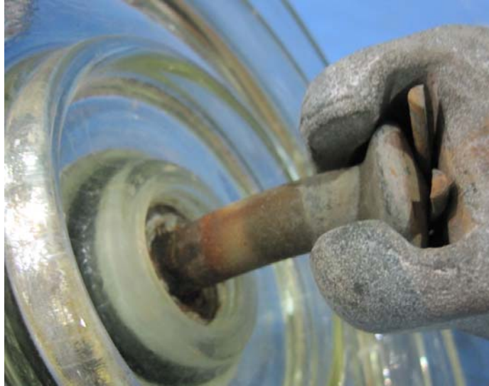
Figure 8 Typical Insulator Sample as received, Bottom View, with Bent Pin (not suitable for Mechanical Testing)
