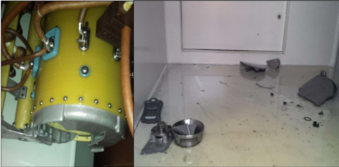
Figure 5: Damaged Tap Changer
