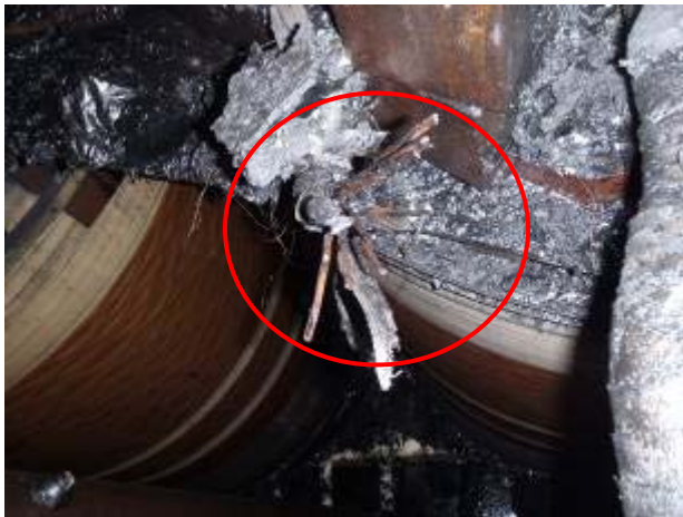
Photo 19 – LV2 Winding Lead Broken
