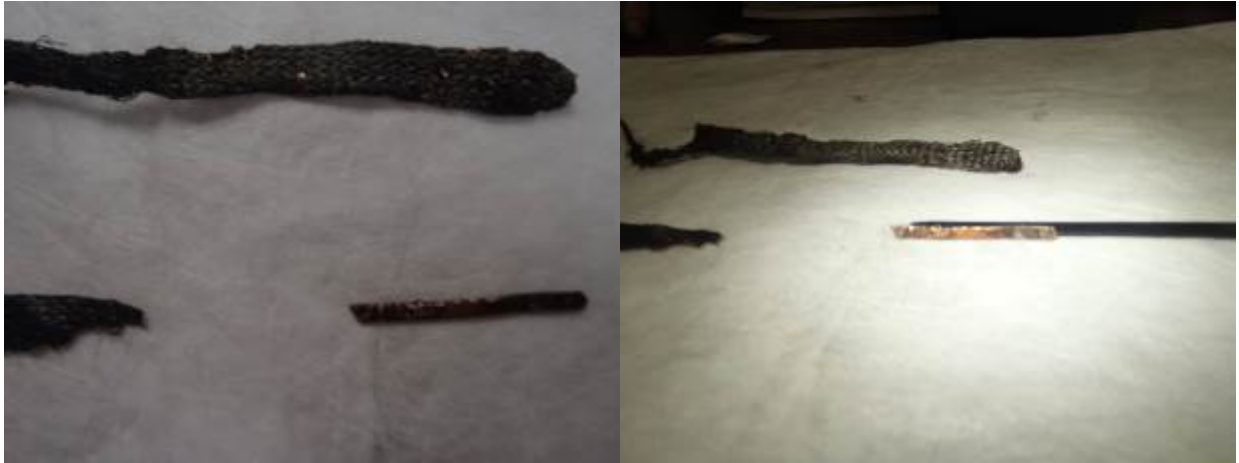
Photo 23 – LV1 Winding Conductor Strand Copper Spitting
