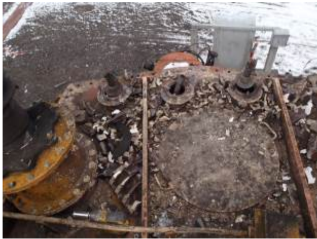
Photo 3 – Cover Open & Broken Bolts
