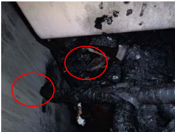
Photo 21 – LV1 Winding Lead Broken
