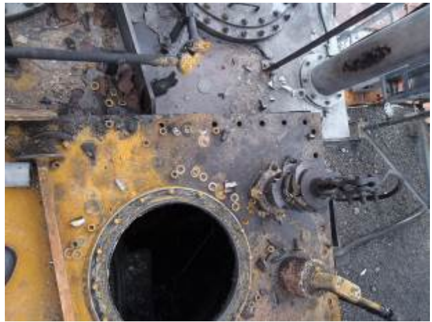
Photo 4 – Cover Open & Broken Bolts
