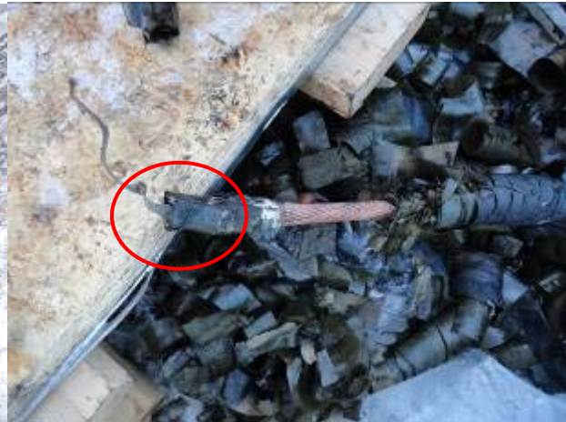
Photo 20 – LV2 Bushing Lead Broken at the Crimp
