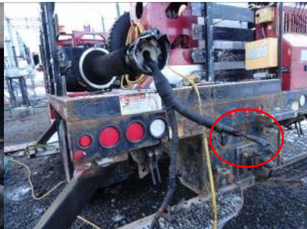
Photo 22 – LV1 Bushing Lead Broken at the Crimp
