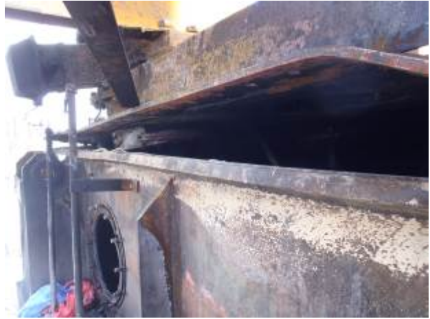
Photo 2 – Cover Open & Broken Bolts
