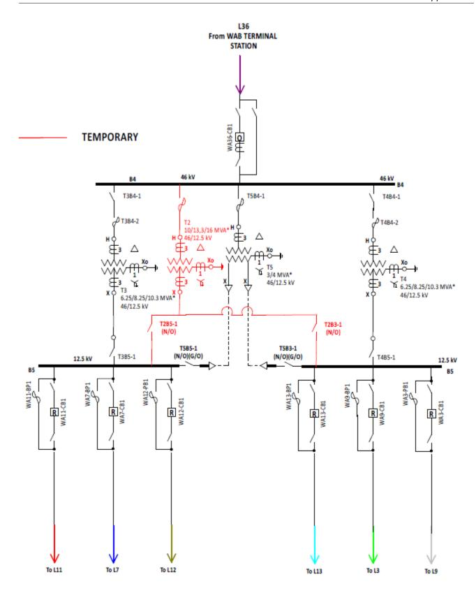
Note 1: Switches T2B5-1 and T2B3-1 must not be closed at the same time
