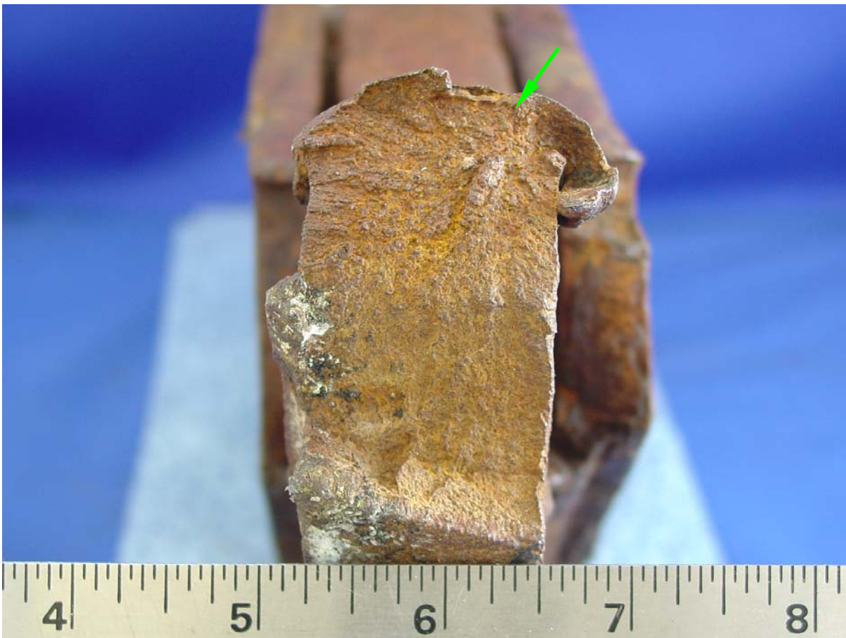
Figure 6: Photograph of the main plate fracture surface. The arrow indicates the likely origin location of the fracture. Scale is in inches.
