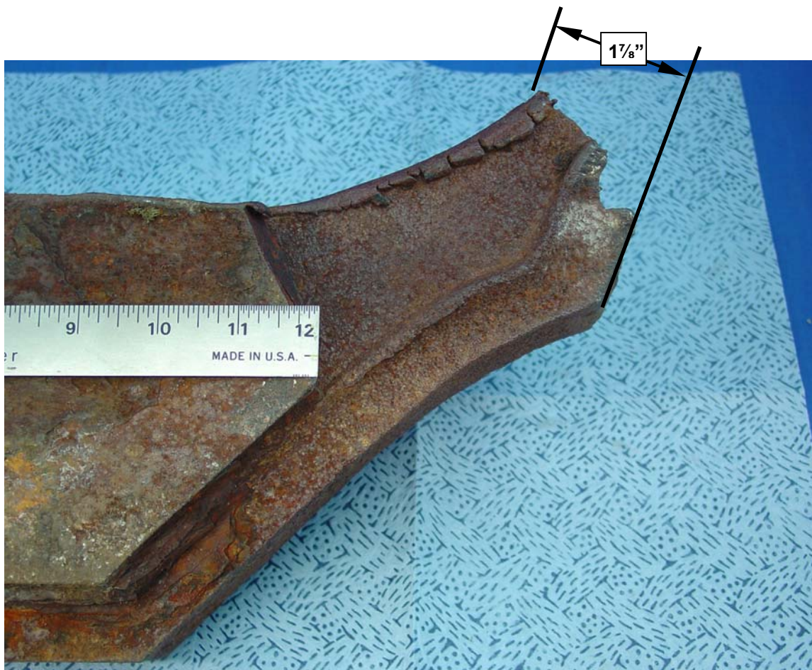
Figure 8: Photograph showing the bottom portion of the hole with dimension lines to indicate how the length of the remaining material was approximated. Scale is in inches.
