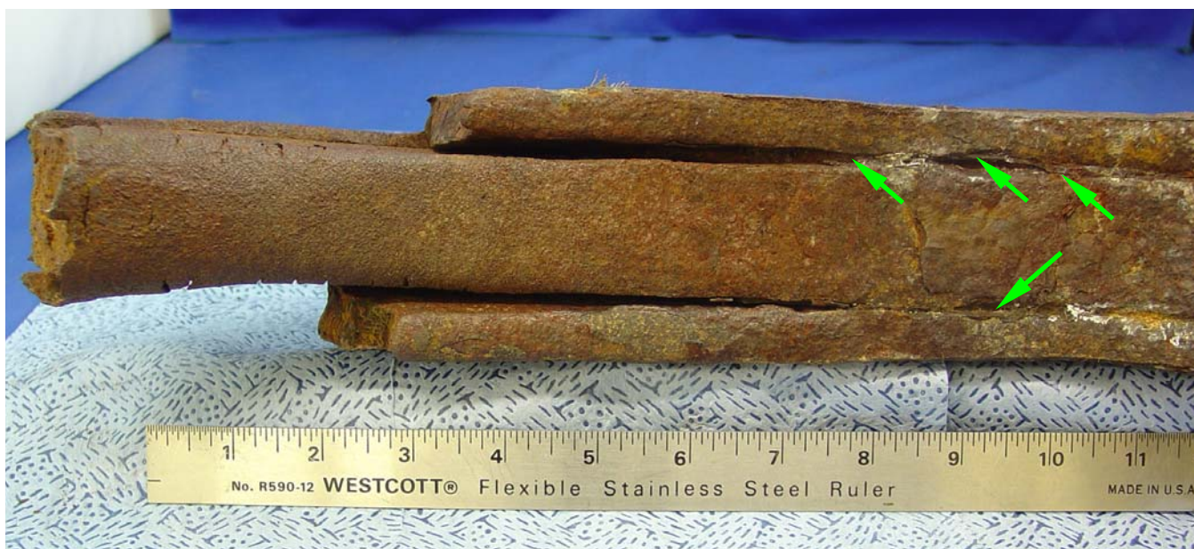
Figure 3: Photograph showing the corrosion between the support plates and the main plate (refer to the arrows) and the gaps that were present between the main plate and the support plates. Scale is in inches.
