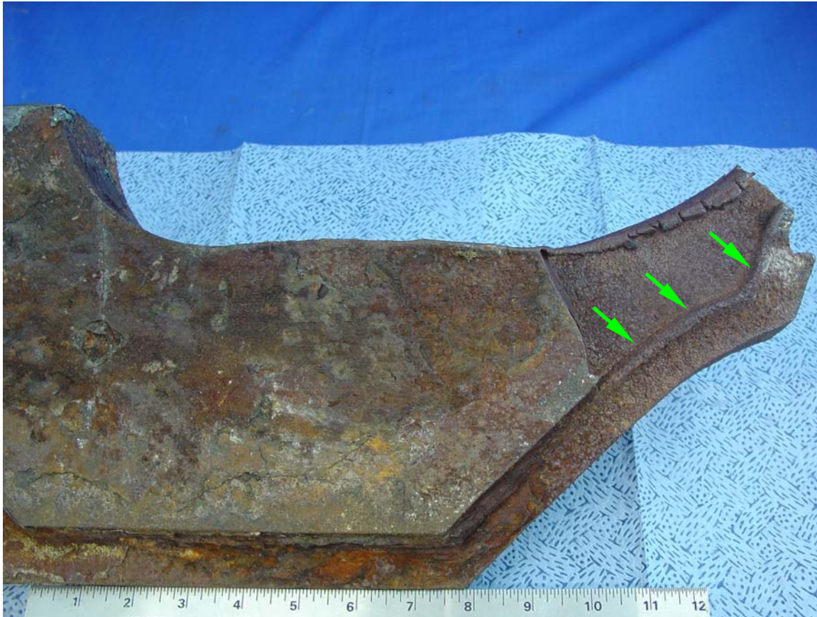
Figure 5: Photograph showing the remnant weld metal on the surface of the main plate (refer to the arrows). Also visible in the photograph is the slight curvature to the diagonal edge of the support arm. Scale is in inches.
