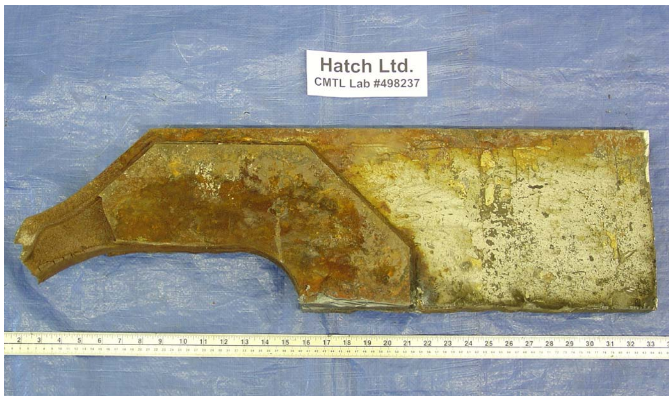
Figure 1: Photograph of the as received section of the marine fender support arm. Top scale on scale marker is in inches and the bottom scale is in centimetres.
