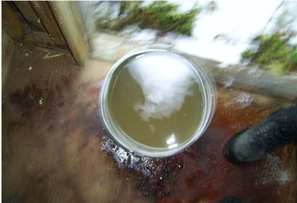
Water quality at outlet – Cloudy with silt and twigs (Site Visit -2)
