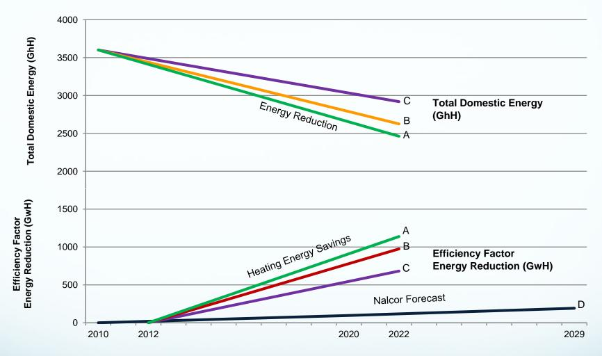
Line A allows for 150,000 electric heated homes converted over 10 years getting 70% reduction for heat (enhanced)
