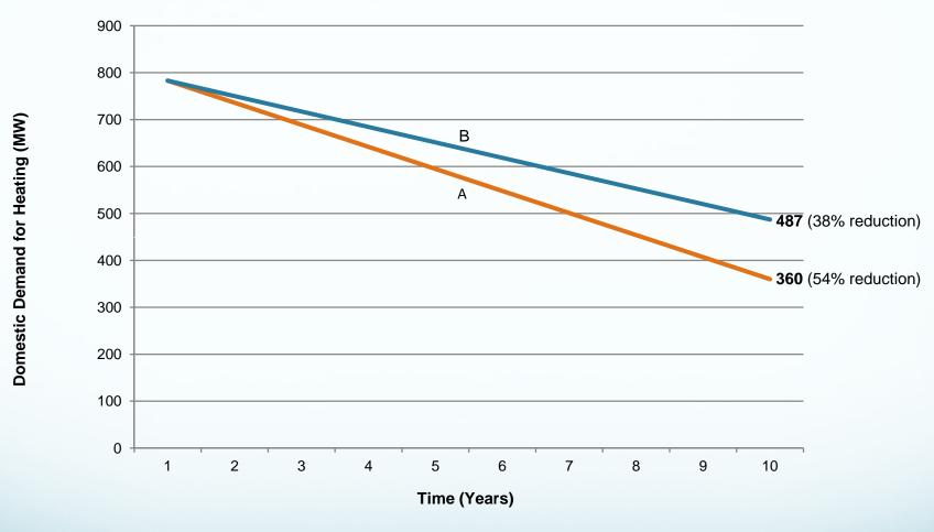
**Line A** Assumes High Efficiency Heatpumps having full coverage gives 423MW reduction **Line B** Assumes High Efficiency heatpumps with 70% coverage gives 296MW reduction
