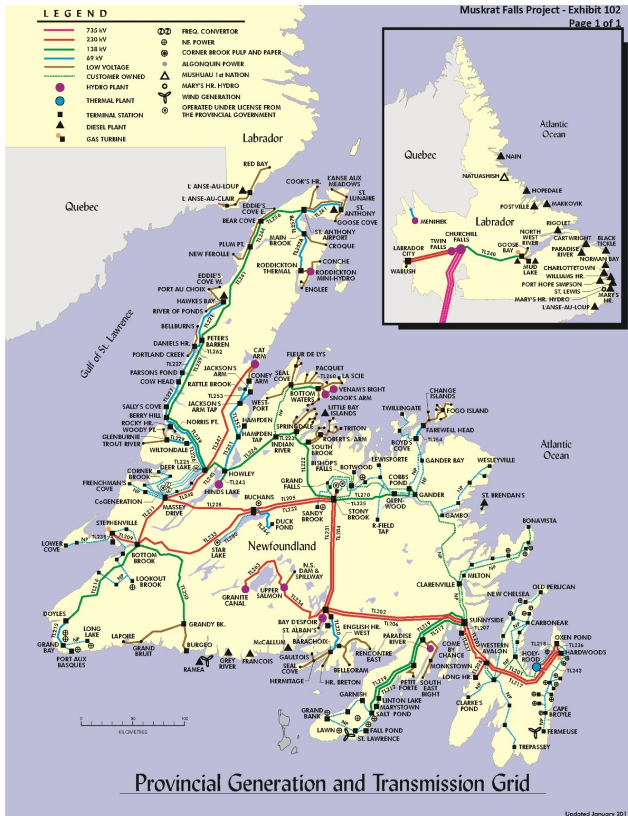
Figure 4: Newfoundland and Labrador Generation and Transmission System Map
