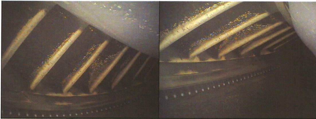
HP NGV,s with pitting and coking
