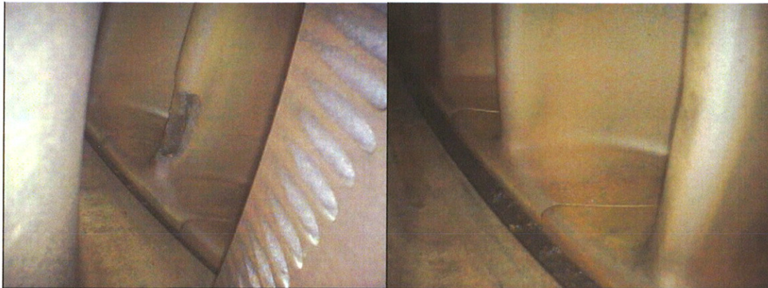
Impact damage on 3 rd blade
