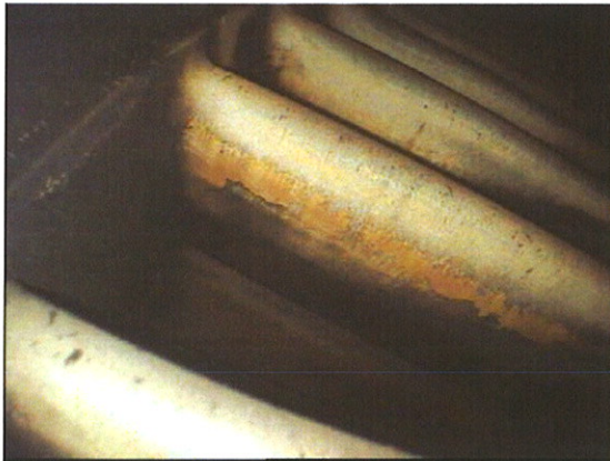
Excessive coating loss on HP NGV
