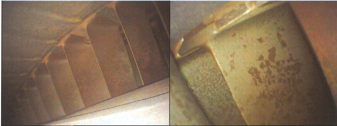
HP Compressor corrosion
