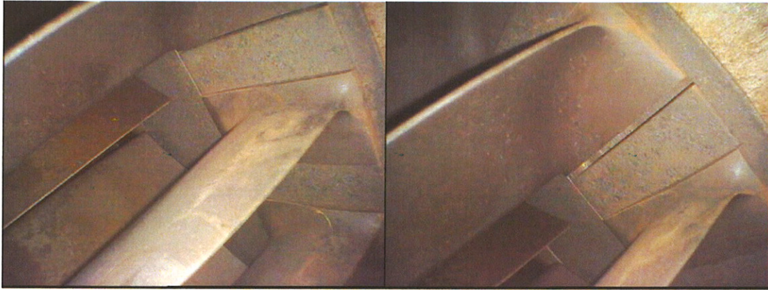
Gap growth on stator
