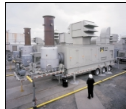
This Cat XQ5200 Mobile Power Unit incorporates gas turbine technology to provide an environmentally friendly power source that can be easily deployed and permitted.
