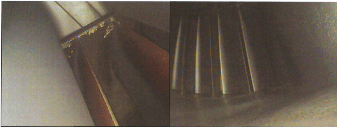
Stage 5 OGV coating loss HP Compressor entries
