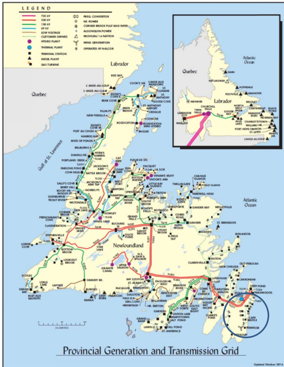
Figure 1: Provincial Generation and Transmission Grid
