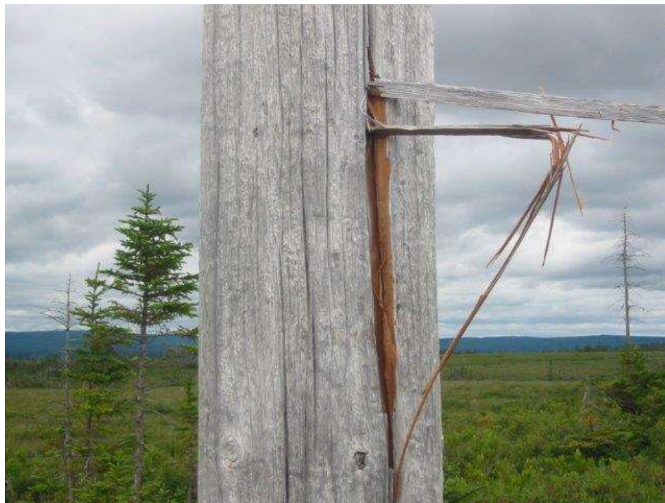
Figure 28 – Pole Shell Separation Showing Exposed Inner Wood
