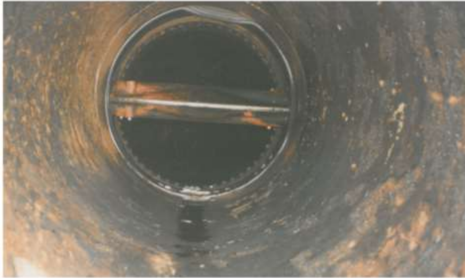
Figure 4 - Main Valve Rubber Seal Separation (Photo Taken in 1991)
