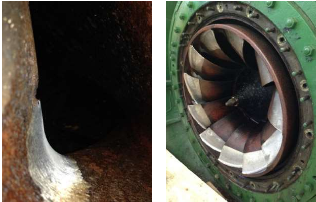
Figure 2 – 2014 Photos of the G2 Turbine Runner Showing High Pressure and Low Pressure Erosion Respectively
