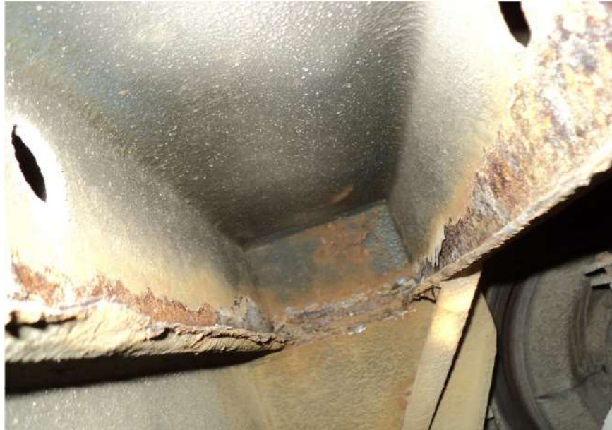
Corrosion on 7" C-Channel
