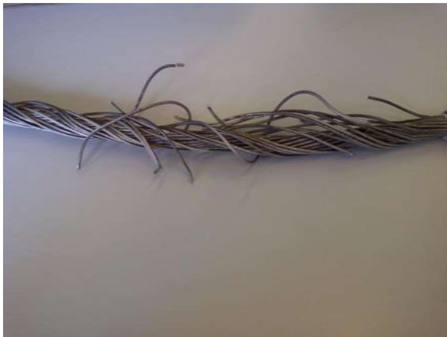
Figure 12 – 18L - Conductor damage removed in 2012
