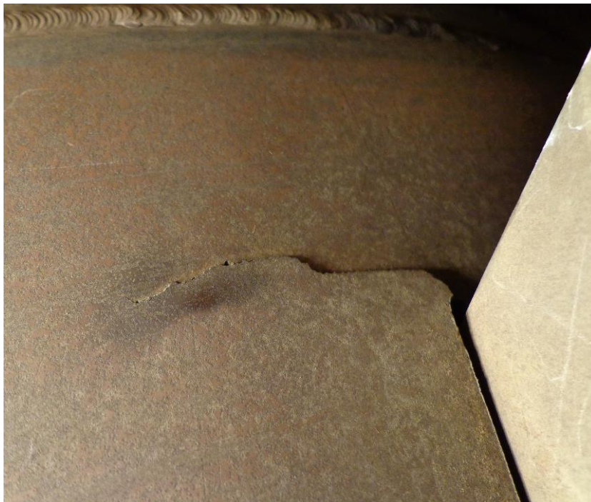
Fig 4 Crack in inner duct
