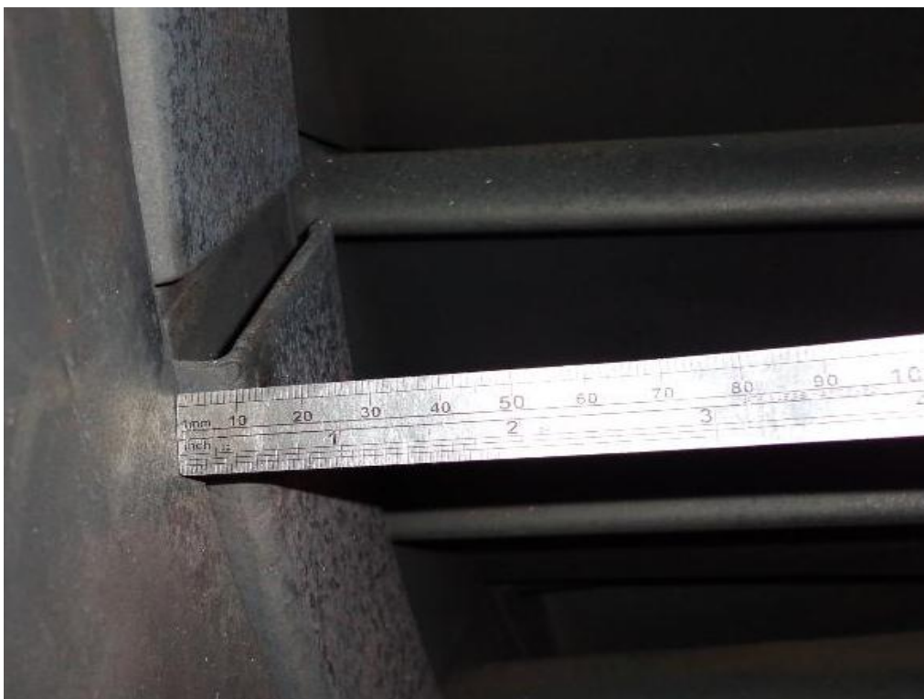
Fig 3 Protrusion of stator shroud
