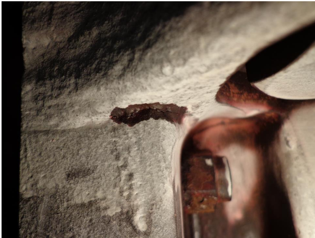
Fig 4 Crack in pressure casing
