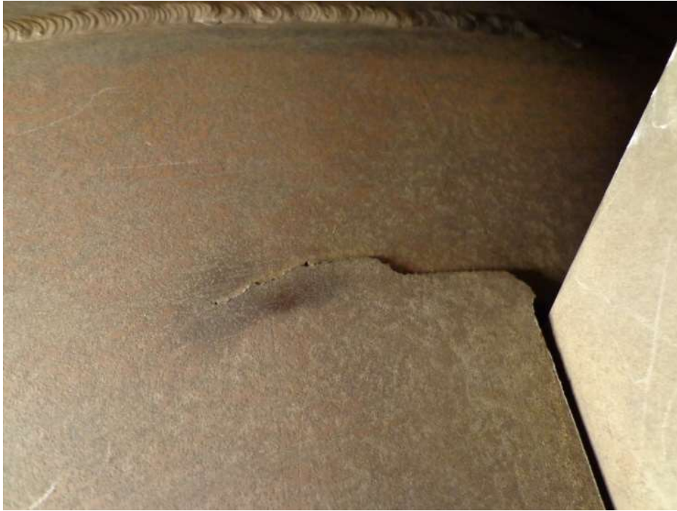
Figure 3 – Crack in Power Turbine Inlet Duct
