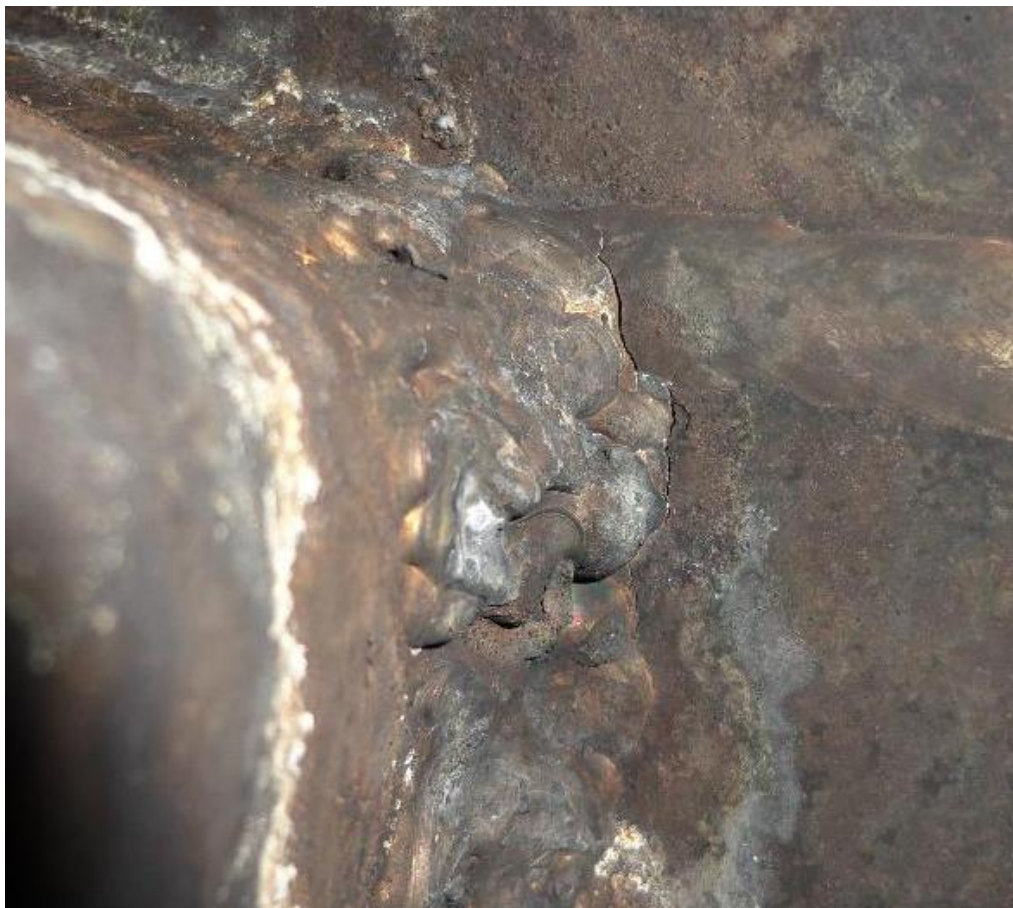
Fig 1 Crack on weld in exhaust.
