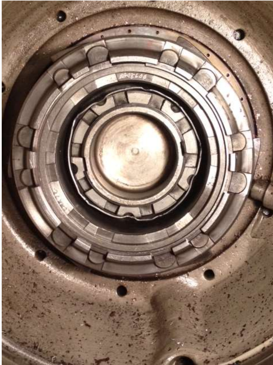
Figure 4 – Damaged Front Bearing
