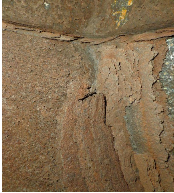
Fig 1 Corrosion in exhaust system.
