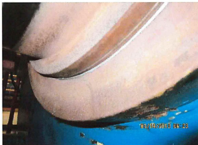
Figure 4 Bearing #4 – lower oil deflector clearance
