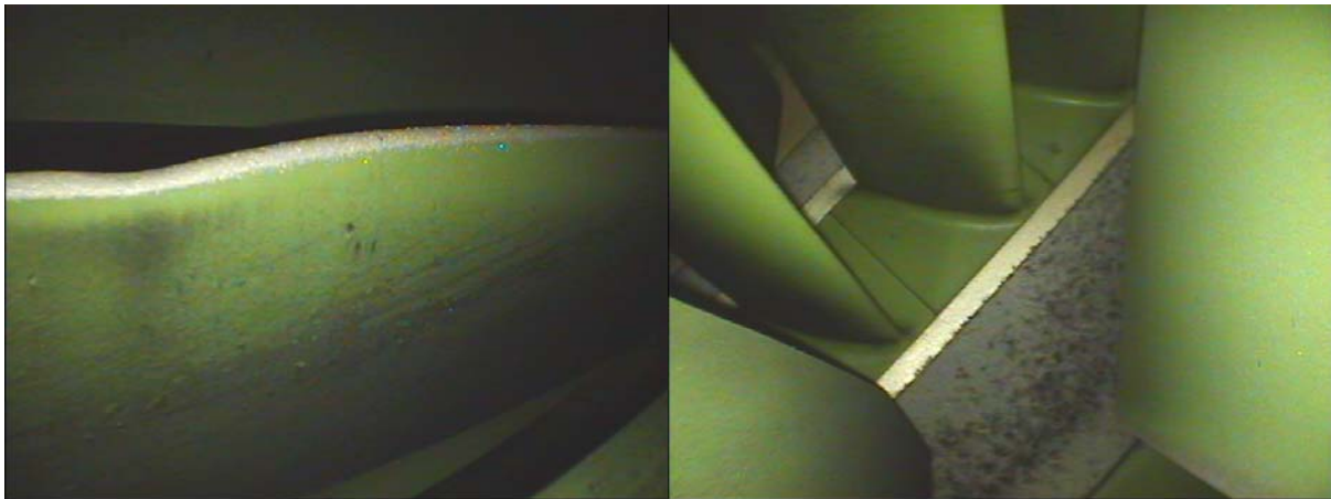
Stage 3 Coating loss and pitting
