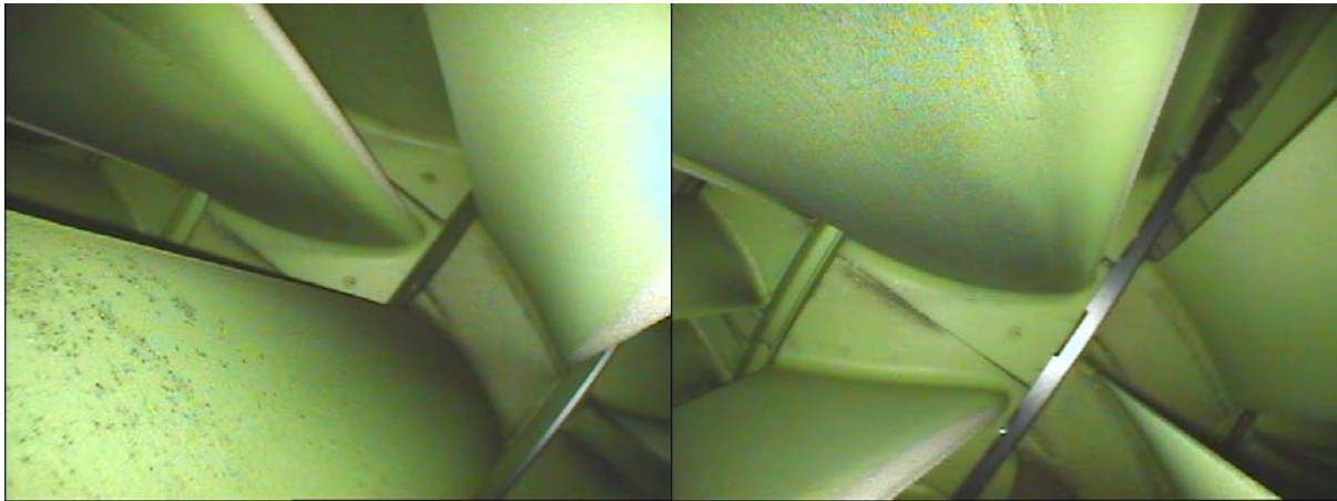
Coating loss and pitting stage 1
