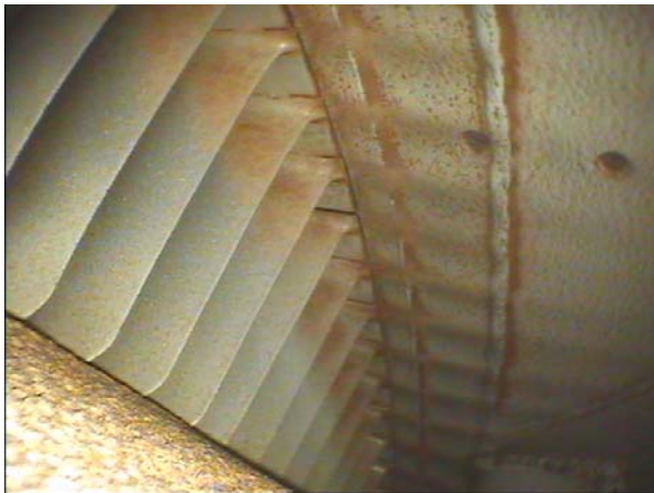
Stage 15 OGV Corrosion
