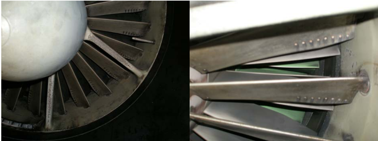
Corrosion pitting on Front Bearing housing struts and outer casing
