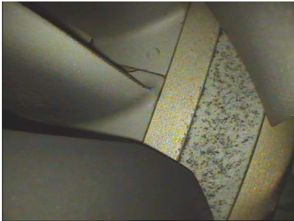
Stage 5 Disc Corrosion
