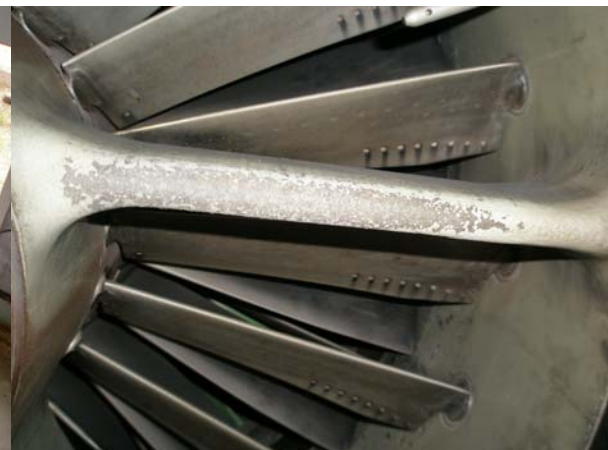
Corrosion on intake
