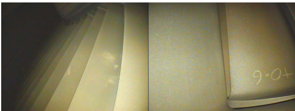
LP Blade coating deterioration
