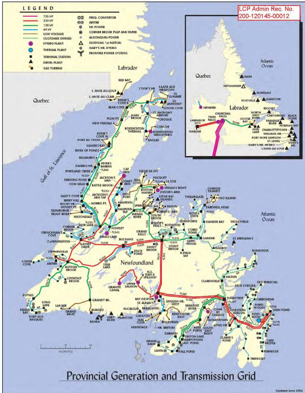
Figure 1-2: Provincial Transmission Grid
