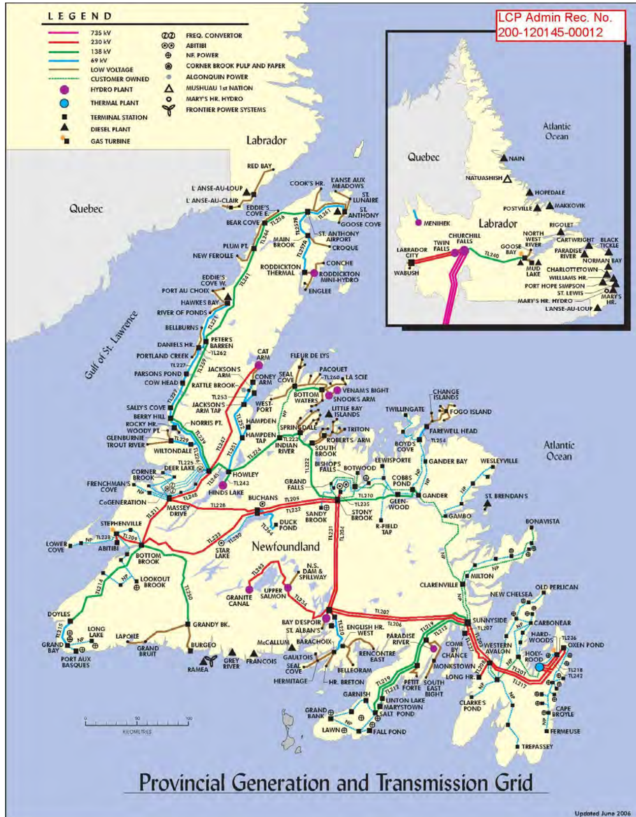
Figure 1-2: Provincial Transmission Grid
