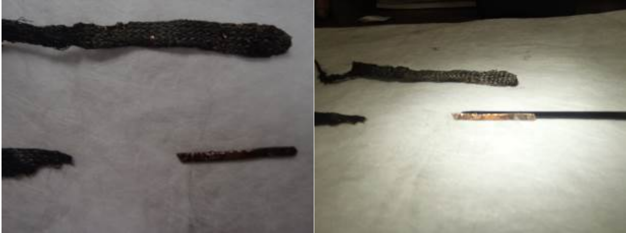
Photo 23 – LV1 Winding Conductor Strand Copper Spitting
