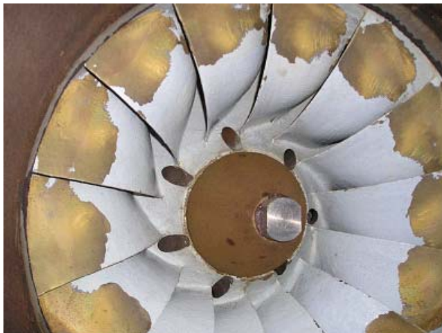
Figure 2-Low pressure side showing loss of belzona coating
