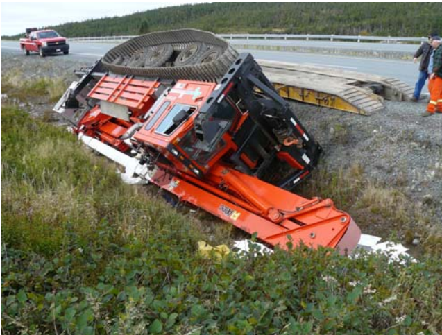
Figure 1. Go-Track unit resting on damaged outriggers and boom.
