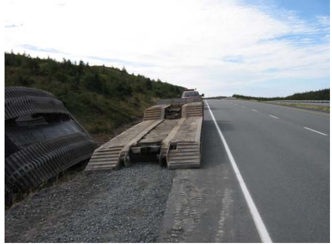
Figure 2. Low bed trailer parked close to the edge of the ditch to maintain clearance to the driving lane as Go-Track unit overhangs trailer deck on both sides when loaded. Note the tilt of the trailer and the shape of the tracks on the Go-Track unit.
