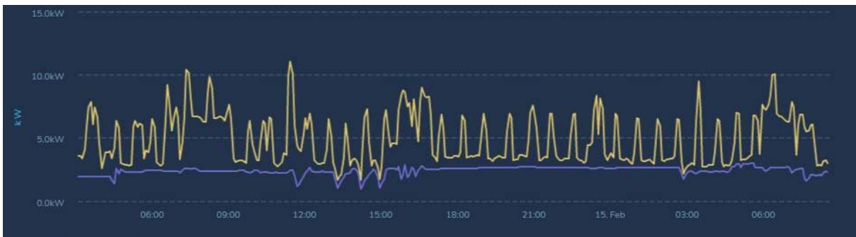
Figure 17: Example DHP with Rapid Oscillations
