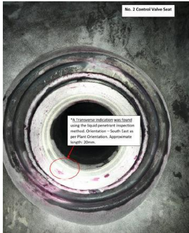
Figure A-3: Crack Found in Control Valve Seat
