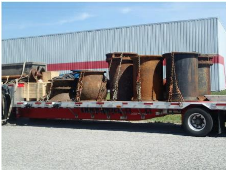
Figure 2: Unit 3 West Cooling Water Pump Shipped to Pump Service Provider Shop in 2017 for Planned Overhaul
