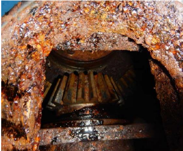
Figure 17: Transfer Case Corrosion – Burnt Dam
