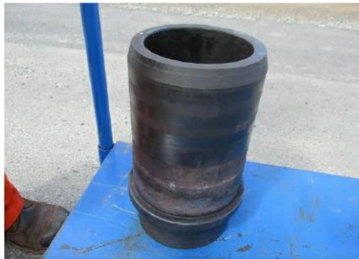
Figure A-4: Failed Control Valve Seat Removed for Replacement
