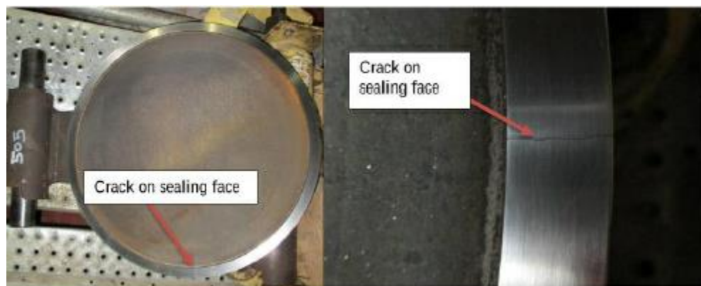
Figure A-1: Crack Found on Sealing Surface of a Non-Return Valve Disc
