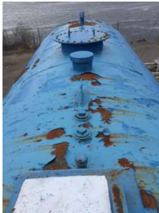
Figure 2: Failed Epoxy Coating and Rust on Tank (Top View)
