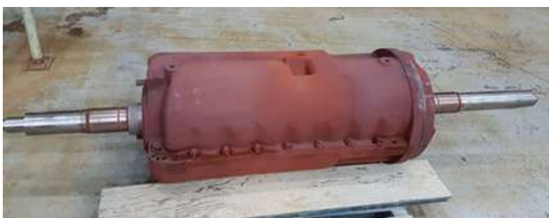
Figure 2: Refurbished Volute Impeller Cartridge.
