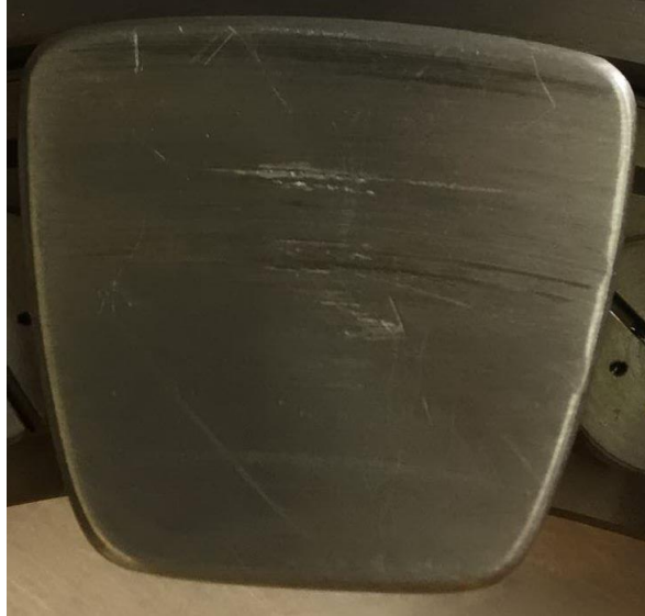
Figure 9: Thrust Pad Wear
