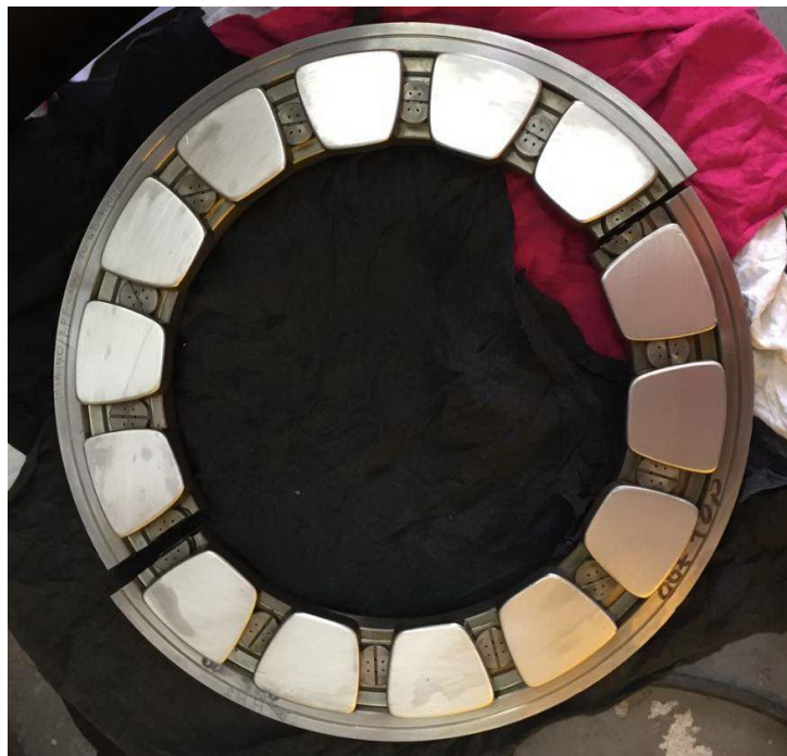
Figure 8: Polished Thrust Ring Prior to Reinstallation
