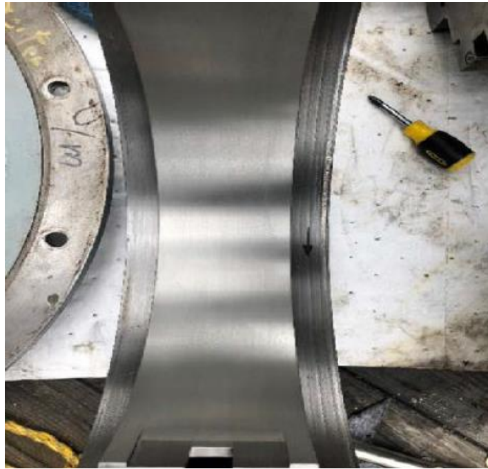
Figure 7: New Exciter Bearing Liner Lower Half Prior to Installation
