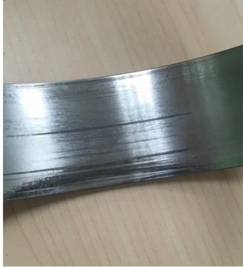
Figure 2: Exciter Bearing Liner Lower half, as Found
