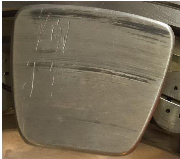
Figure 10: Thrust Pad Wear
