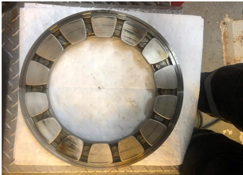
Figure 5: Exciter Bearing Thrust Ring A Side, as Found
