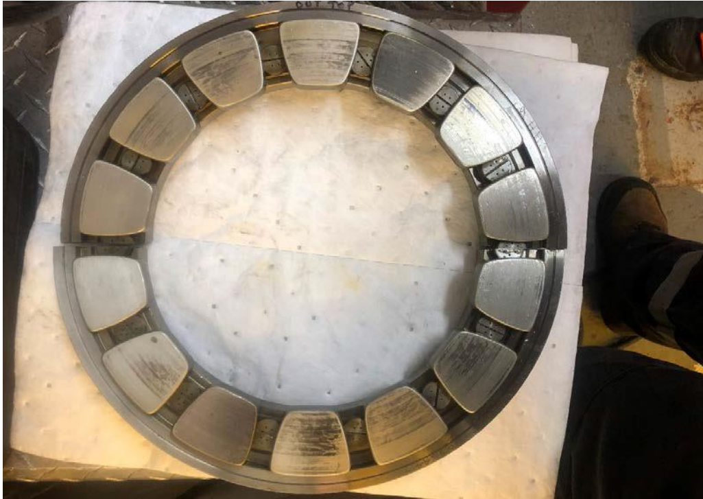
Figure 4: Exciter Bearing Thrust Ring B Side, as Found
