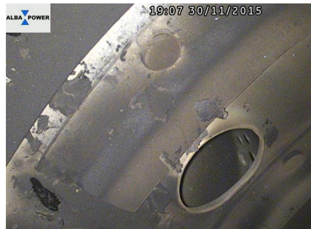
Carbon build up on combustion chamber
