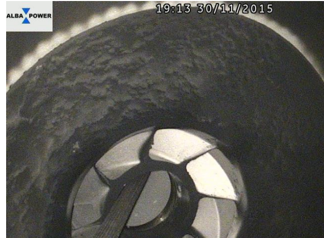
Carbon build up on base of combustion can
