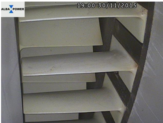
Rear stages of HP compressor
