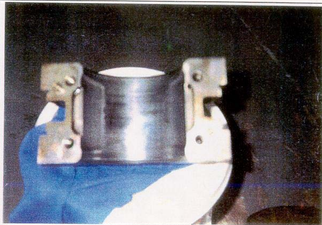
Photo 4: Shows scoring that has occurred on the pedestal bearing which has failed - August 19, 1998
