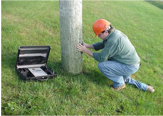
Figure 3.4c - PoleTest in Use
