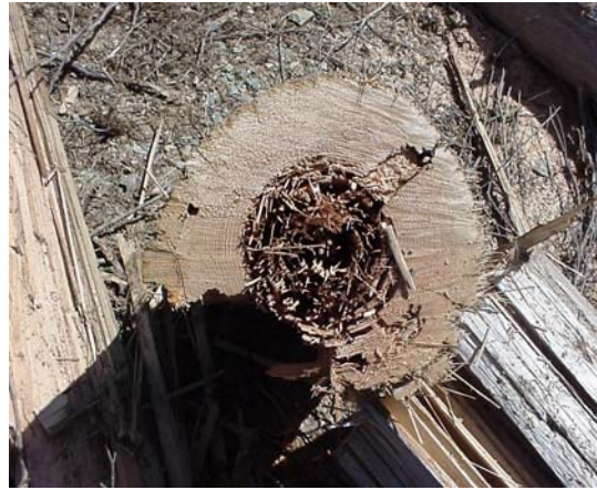
Fig. 3.19b – Carpenter Ant Damage
