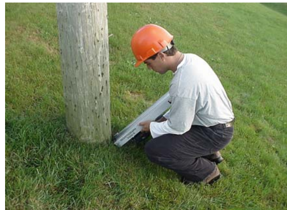
Figure 3.4b - Resistograph in Use
