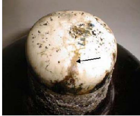
Fig. 3.22b – Cement Crack (CEA, 2003)
